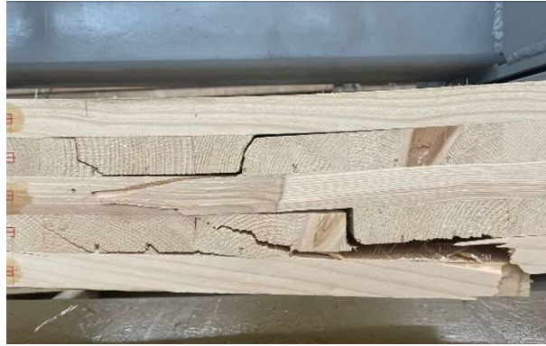
Fig. 8 Typical failure mode of Series A panels (specimen A1)
